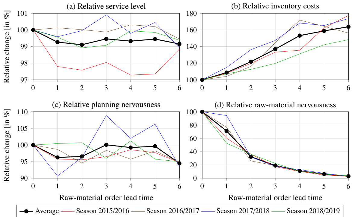
Figure 5: Sensitivity analysis of raw-material ordering lead time.
